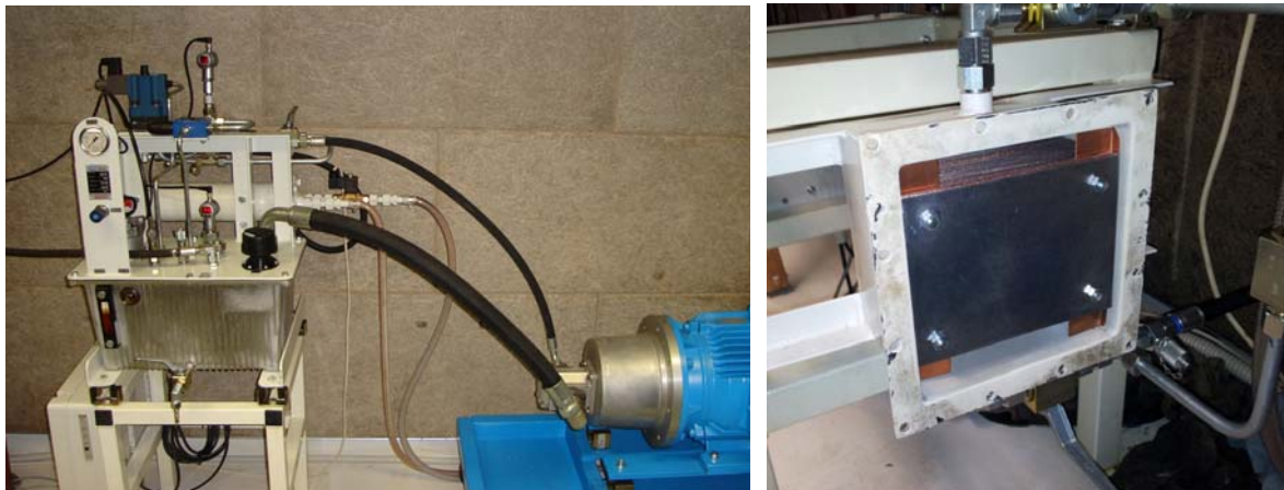
Figure 2. Special test unit for mechanical oil-ageing testing (left) with the catalytic unit (right).
