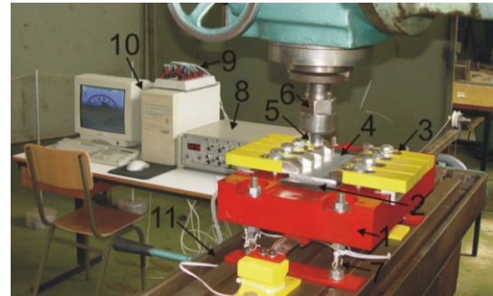
Figure 3. Research site: 1 - The base plate, 2 - Support plate, 3 - Workpiece clamp, 4 - Workpiece of Al alloys, 5 - Tool for FSW, 6 - Clamp part of the milling machines, 7 - Special carrier with glued strain gauge, 8 - Measuring bridge, 9 - BAS, 10 - PC with A/D card and software for data acquisition, 11 - Work table of milling machine [3, 4]
