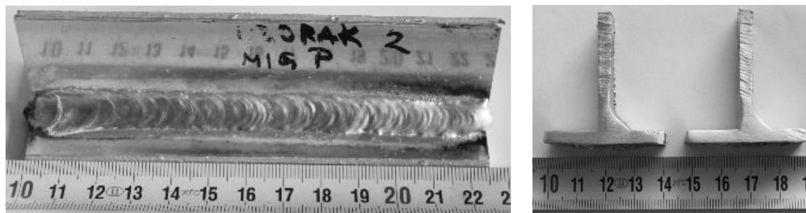
Figure 2. Welded sample (left) and sample after cutting for macroscopic evaluation (right)
