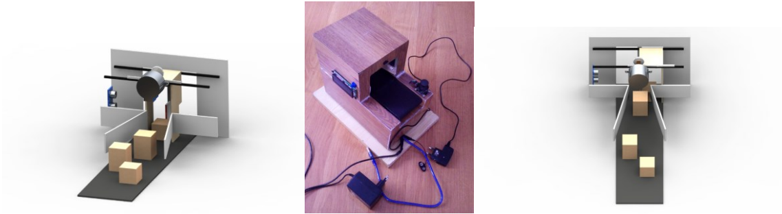
Figure 4. 3D and physical model of the conveyor belt
