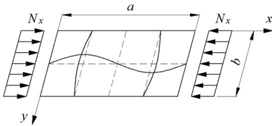
Figure 1. Buckling of simply supported, uniformly compressed rectangular plate
