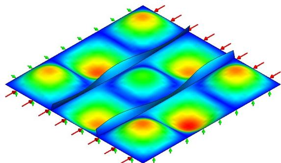
Figure 4. Local buckling mode of the steel stiffened plate ( $a \times b \times t = 1500 \times 1500 \times 7$  mm,  $t_s \times b_s = 8 \times 62$  mm)
