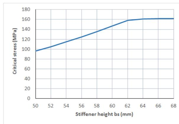
Figure 6. Graphical representation of the influence of flat stiffener height  $b_s$  on the critical stress ( $a \times b \times t = 1500 \times 1500 \times 7$  mm,  $t_s = 8$  mm)
