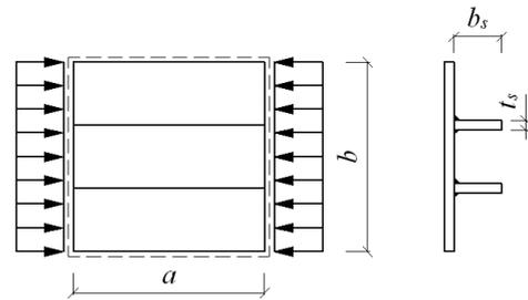
Figure 2. The layout of the stiffened plate
