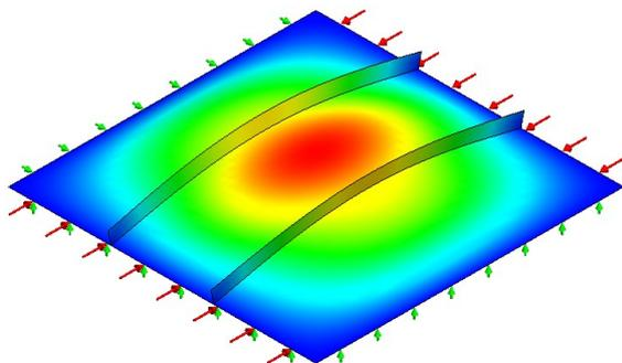
Figure 3. Global buckling mode of the steel stiffened plate ( $a \times b \times t = 1500 \times 1500 \times 7$  mm,  $t_s \times b_s = 8 \times 60$  mm)
