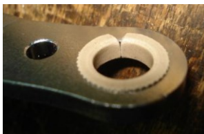
Figure 1: Bushing assembled on Lever
